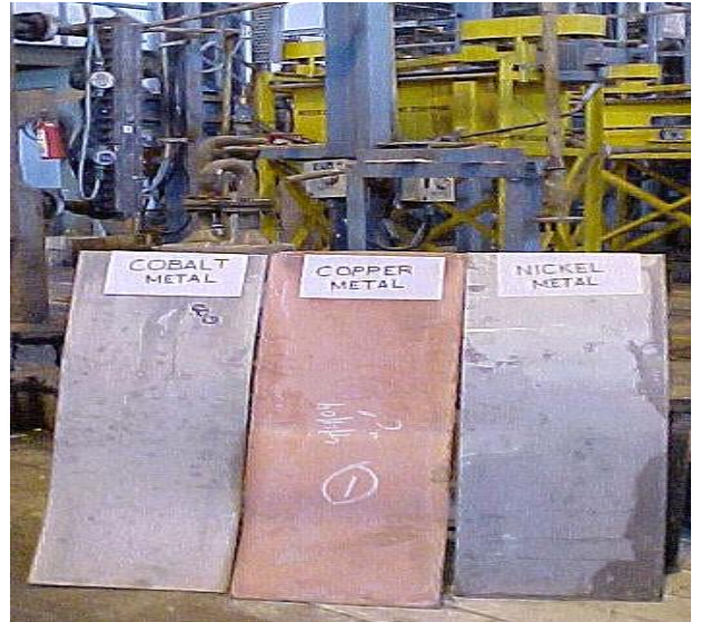
High pure Co, Cu and Ni metal cathodes produced from low grade resource
