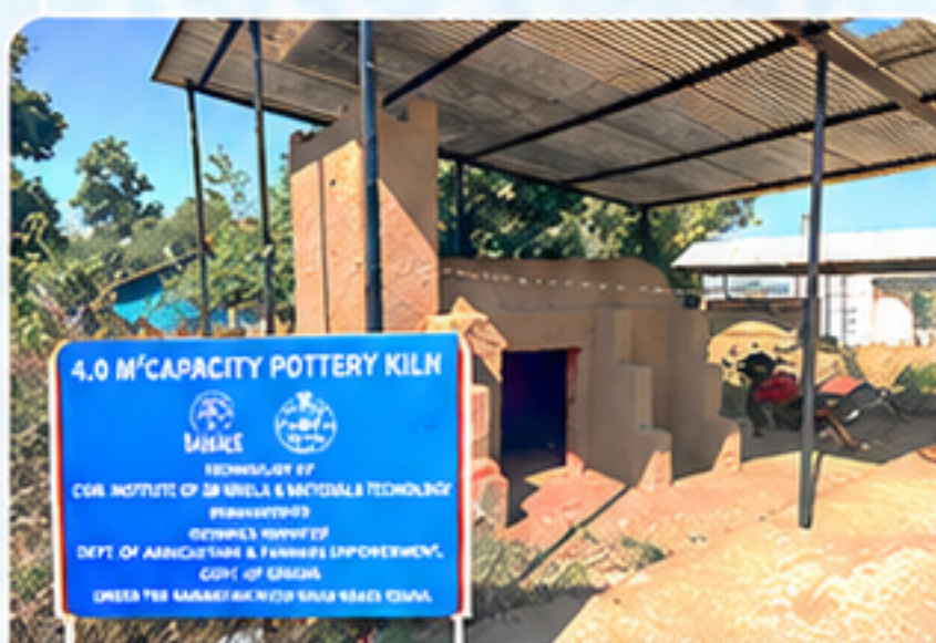
Terracotta Sintering through Improved Kiln
