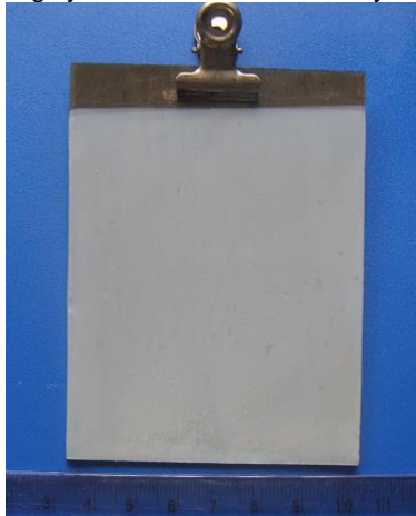
Highly adhered \text{TiO}_2 on steel by EPD
